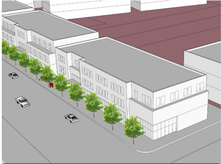
These conceptual models illustrate both building articulation along the street, and modified upper story height using a setback.
