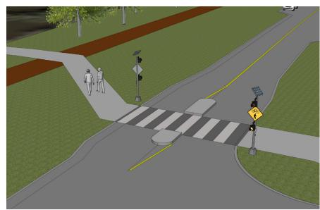
Figure 5.14: An RRFB signal and small median island are proposed to create a safer crossing of Ellicott Creek Road at Thistle Avenue.
