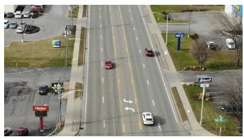
Figure 4.13: Frequent curb cuts and the continuous center turn lane creates numerous conflict points for all roadway users (pedestrians, cyclists, and vehicles).
