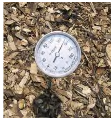
Thermometer showing elevated temperatures.
