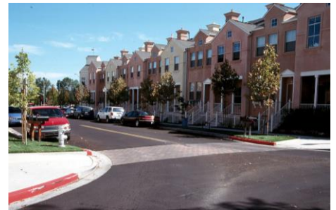
An example of traffic calming measures, such as reduced lane width, crosswalk, landscaping, and on-street parking.
