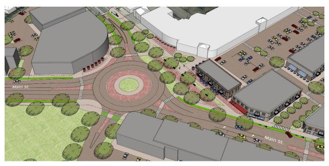
Figure 6: Birds-eye view of Option 1 for the intersection of Main Street, Kenmore Avenue and the new South Campus entrance alternative with roundabout (requires further study)
