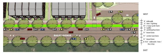
Figure 4: The proposed improvements along Bailey Avenue between Sherman Road and Main Street include infill graduate student housing, improved pedestrian connections into the campus, sidewalks with street trees and site furniture, and a separated two-way cycle track.
