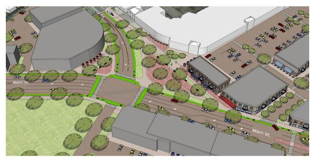
Figure 7: Birds-eye view of Option 2 for the intersection of Main Street, Kenmore Avenue and the new South Campus entrance alternative with enhanced pedestrian/bike crossings and traffic signals with pedestrian scramble phase
