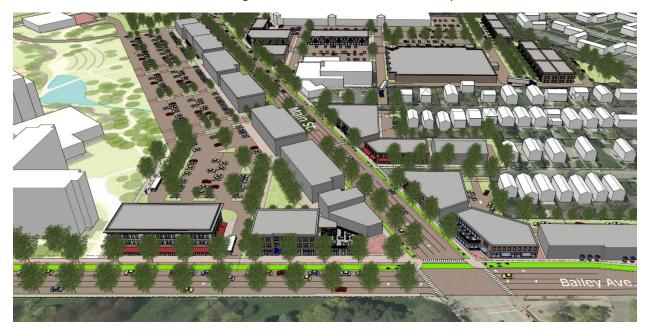
Figure 3: Birds-eye view of the intersection of Main Street and Bailey Avenue showing the proposed protected cycle tracks
