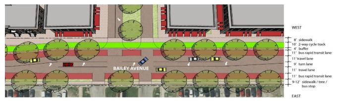
Figure 5: The proposed improvements along Bailey Avenue between Winspear Avenue and Sherman Road include infill mixed-use buildings with parking in the rear, improved pedestrian connections into the campus, sidewalks with street trees and site furniture, a separated two-way cycle track, and bus rapid transit lanes.
