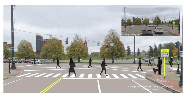
Figure 8: Illustration of the pedestrian scrabble concept at the intersection of Main Street, Kenmore Avenue and the new South Campus entrance, looking towards the campus (illustration by GBNRTC)
