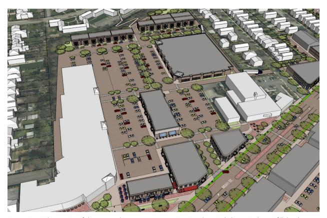
Figure 13: Birds-eye view of the proposed improvements at University Plaza, including mixed-use infill development along Main Street, streetscape improvements, and better organization of building masses, pedestrian spaces, pedestrian connections and vehicular circulation.
