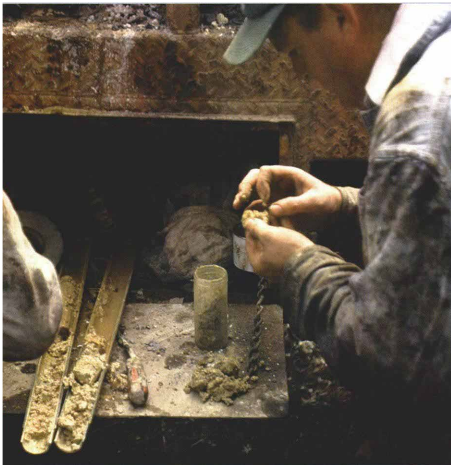
Not exactly wine tasting. Soils engineers inspect core samples they've taken using the split-barrel sampler on the left.
