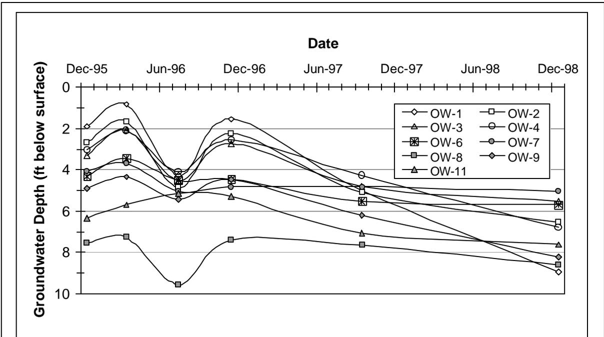
**Figure 15. Groundwater levels in shallow wells at Spaulding Site, north of former Tonawanda Landfill (see Appendix 6.1.4). The midpoint of the sandpack for all wells is about 14 feet below ground surface in silty clay (probably till). Data shows spatial and temporal variability in shallow groundwater level. (Data source: Glen May, NYSDEC, 2005)**
