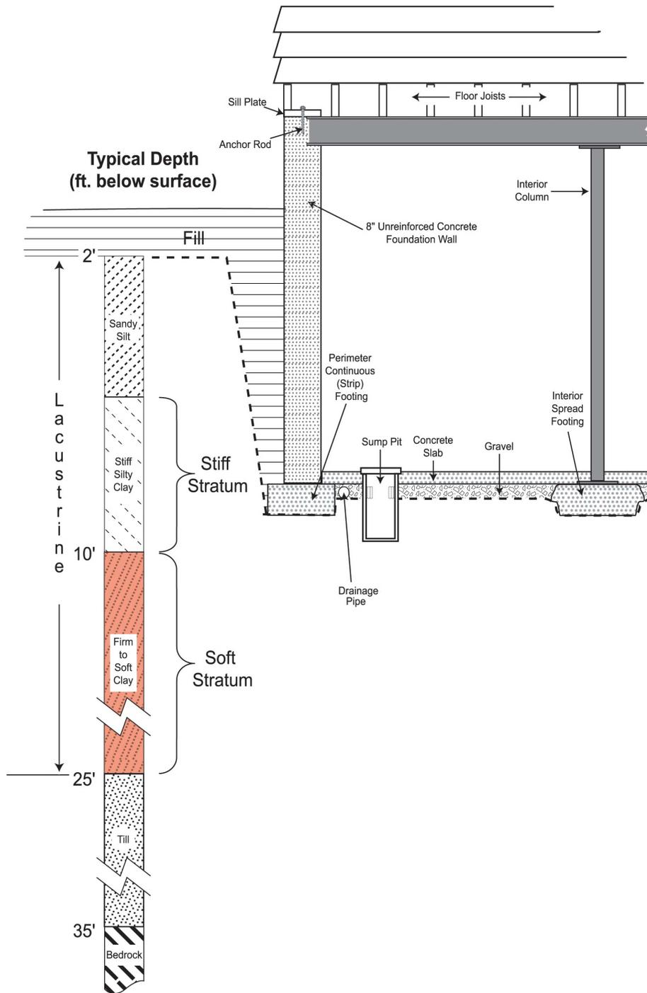
**Figure 8. Schematic stratigraphic soil profile in central and northern Amherst showing typical construction of older houses. Many footings rest on a stiff stratum that overlies a soft stratum. Fill consists of remolded native material.**
