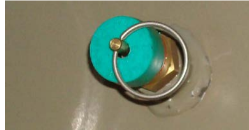
Figure 4. Automatic pressure relief valve
