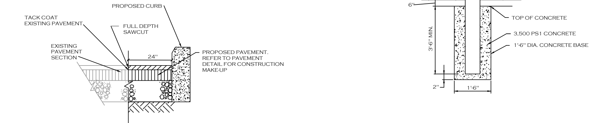
CURB AND PAVEMENT TRANSITION DETAIL
