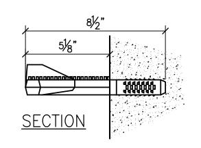
MANHOLE STEP DETAIL SCALE : 3'' = 1'-0''
