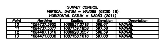
NOTE: UNITS USED TO PREPARE THIS MAP ARE BASED ON THE U.S. SURVEY FOOT.
