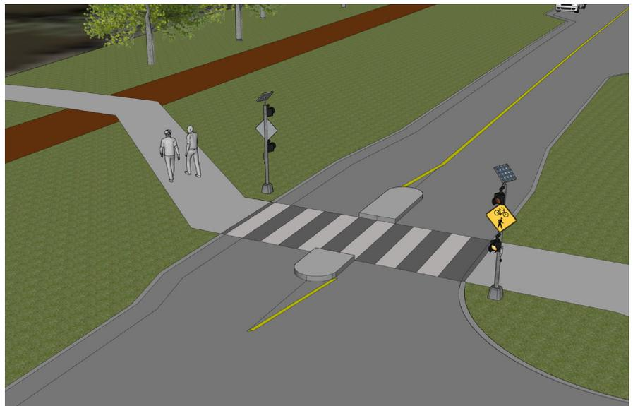
Figure 5.14: An RRFB signal and small median island are proposed to create a safer crossing of Ellicott Creek Road at Thistle Avenue.
