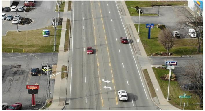
Figure 4.13: Frequent curb cuts and the continuous center turn lane creates numerous conflict points for all roadway users (pedestrians, cyclists, and vehicles).
