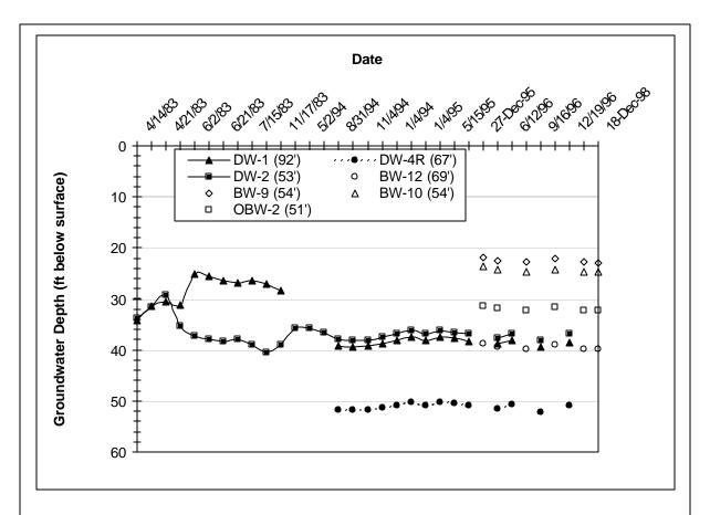
Figure 20. Hydrograph of till (open) and shale (solid) monitoring wells at the Tonawanda landfill. NY. Legend indicates midpoint depth of screened interval (see Appendix 6.4). Note hiatus in dates. (Data source: Glen May, NYSDEC, 2004)
