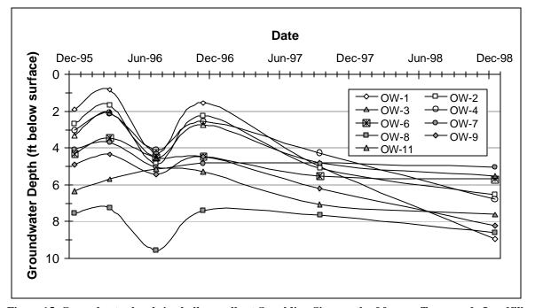
Figure 15. Groundwater levels in shallow wells at Spaulding Site, north of former Tonawanda Landfill (see Appendix 6.1.4). The midpoint of the sandpack for all wells is about 14 feet below ground surface in silty clay (probably till). Data shows spatial and temporal variability in shallow groundwater level. (Data source: Glen May, NYSDEC, 2005)
