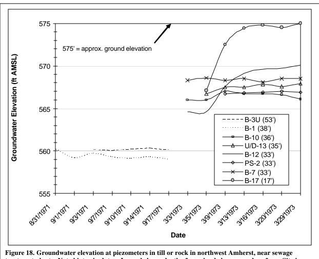
treatment plant. Note hiatus in dates. Legend shows depth of opening below ground surface. Site is nearly flat with ground elevation ~ 575 ft AMSL. (Data source: Ward, 1971 & 1973).
