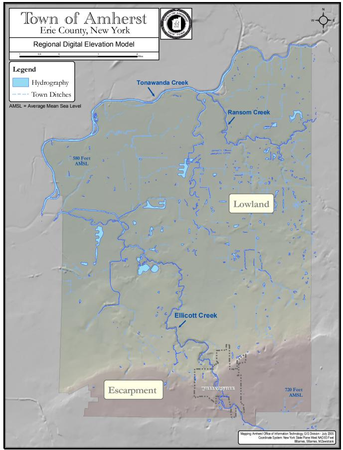
Figure 2: Digital elevation model (DEM) of Amherst, NY, showing change in relief from escarpment to lowland areas.
