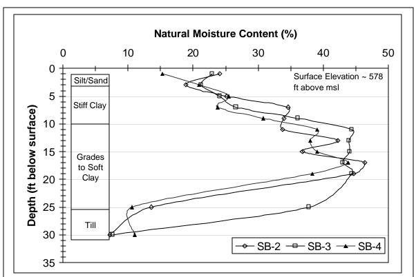
Figure 9. Typical soil moisture content profile from three soil borings at sewage treatment plant in northwestern Amherst. Data from Ward (1973).
