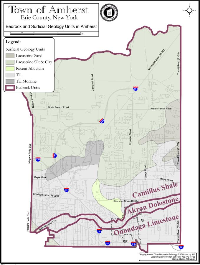
Figure 4: Surficial and bedrock geology of Amherst, NY. Lacustrine deposits (north) and till (south) overly gypsiferrous shale and calcarious rocks (dolostone and limestone) respectively (Source: NYSGS, 2005).
