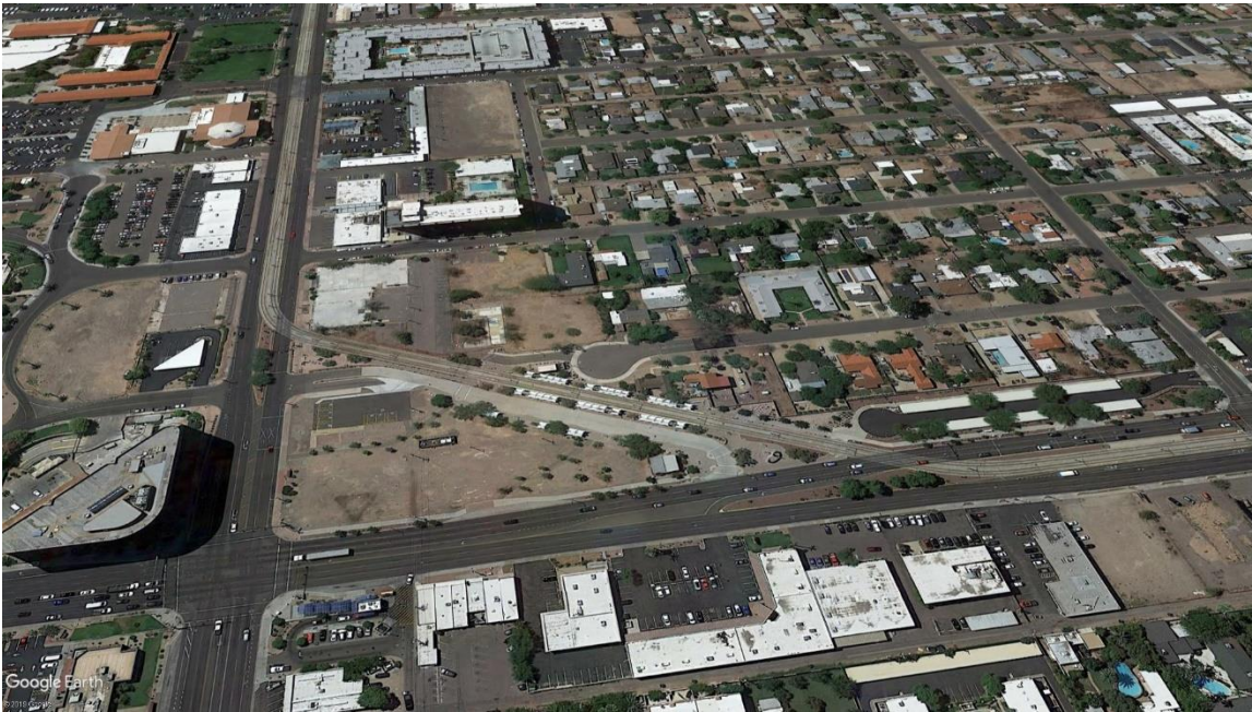
Example Cut-Through Light Rail Turn in Phoenix, Arizona
