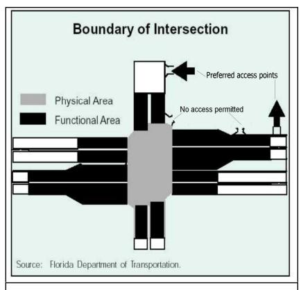
Figure IV-1: Illustration of the functional area of an intersection and the preference for points of access to be located outside the area. (Source: Florida Department of Transportation)
