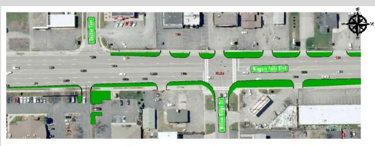
Figure 10: Willow Ridge Drive Intersection Narrowing (Option A)
